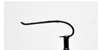
1. Pinch the barb, place the hook in the vice, start the thread and wrap to between the barb and the point of the hook.
